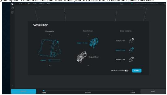
Here you can choose your printer/machine (we keep adding new ones) and tool head, which will also affect the specific workflow you will be using: 3D printing, CNC, Laser or thick paste extrusion.
