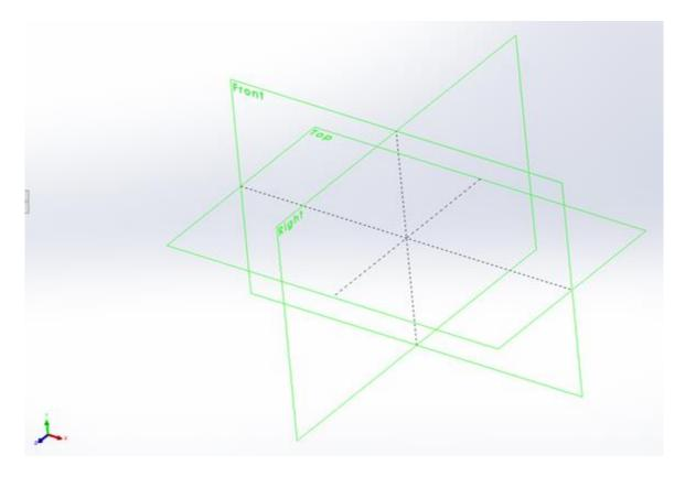
And final important entity of our 3D space is the origin, the point that is in zero coordinate, many times used as a main coordinate reference for each of the directions and is widely used in dimensioning.
