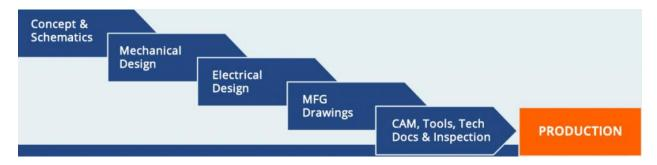
**Concept design** - where the product is defined by its properties and tasks, especially if the exterior is important then concept sketches are made
