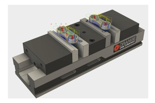
When a design is complete in CAD, it can then be loaded into CAM. This is traditionally done by exporting a CAD file and then importing it into CAM software. If you're using a tool like Fusion 360, both CAD and CAM exist in the same world, so there's no import/export required.
