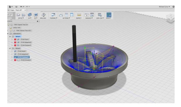
Once the model is prepared for machining, all information is sent to a machine to start producing the part physically. However, we can't just give a machine a bunch of instructions in English. We need to speak the machine's language. To do this, we convert all of our machining information to a language called G-code. This is the set of instructions that controls a machine's actions including speed, feed rate, coolants, etc.
