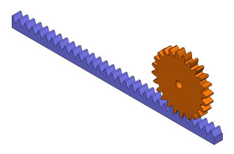
In the example above we see one more gear mechanism where longitudinal movement is transferred into rotational or rotational movement into longitudinal, depending on which side will be the input.
