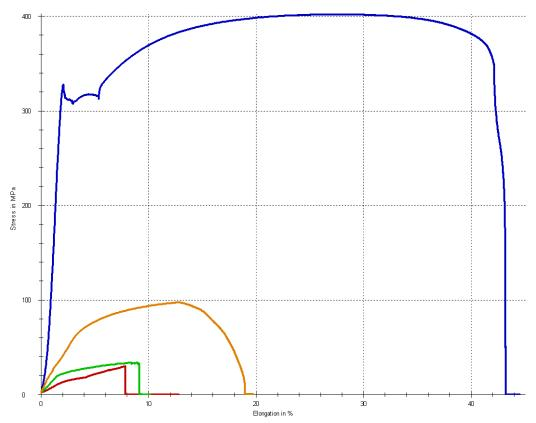
Test curves, from the above-given table you should be able to determine which curve is for which sample, (hint: use the  $R_{max}$  column from the table)
